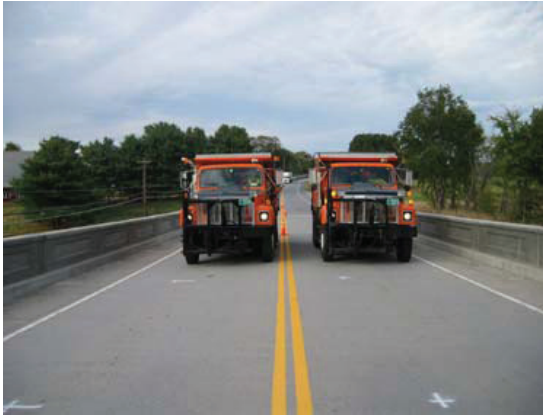
Field testing of the bridge
